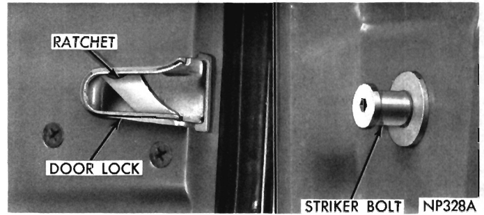
Fig. 14 Door Lock Ratchet and Striker Bolt
